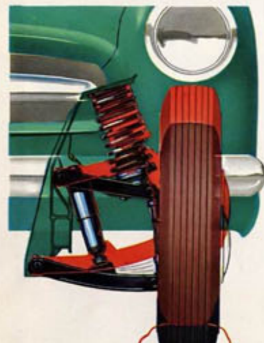
EXCLUSIVE NASH AIRFLEX FRONT SUSPENSION plus low center of gravity and scientific distribution of weight, combine to give the Metropolitan unusual "cornering" stability and ride control.
