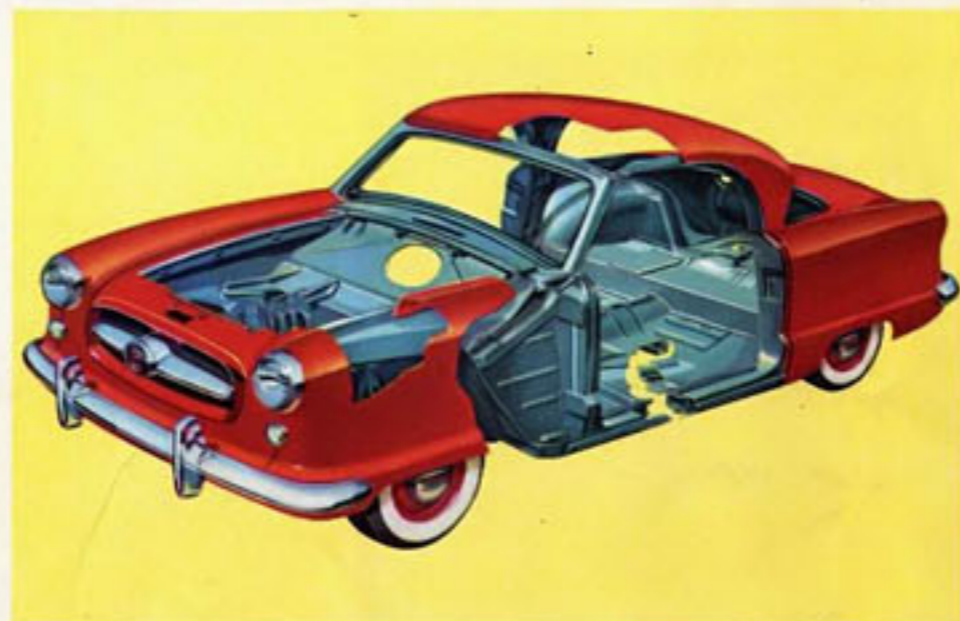
LIFE-SAVING SAFETY of double-rigid Nash Unitized Airflyte Construction gives you sturdiness never before possible in a car of this size. Body-and-frame are welded into a single unit to give you a "double lifetime" of service. Airflyte Construction is stronger, safer . . . lastingly free of body-bolt squeaks and rattles.
