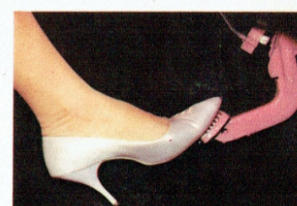
Rambler Step-on Parking Brake is an appreciated convenience feature that is standard equipment on all models. Hand release is located above the foot pedal. Handy warning light is optional.
