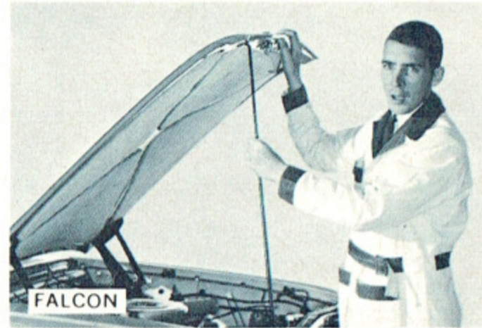
FALCON Contrast Rambler American's counter-balanced hood with the Falcon hood-opening arrangement. The Falcon and Comet still use the old-fashioned prop rod to hold the hood open.
