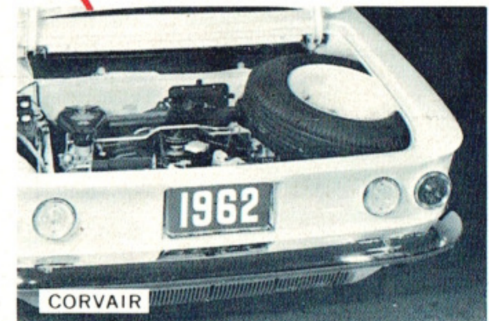
CORVAIR Corvair's spare tire is located above and to the side of the rear engine where the rubber is subjected to engine heat. Rambler American's spare tire is carried conveniently in the trunk.
