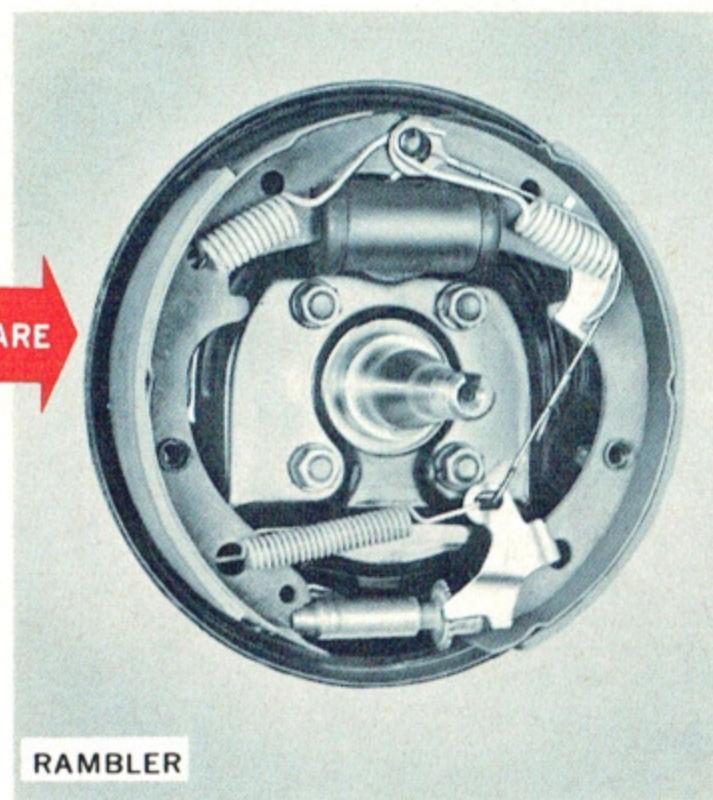
RAMBLER The front hydraulic brake line on the American is similarly cut. But the rear brake line still works to bring the car to a quick, sure stop.
