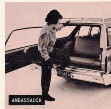
AMBASSADOR Ambassador (and Classic)...convenient side-hinged rear door simplifies entry...makes the optional third seat more accessible for adults.
