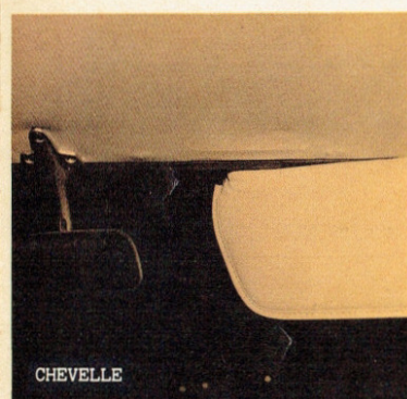
CHEVELLE Chevelle sun visors have no inner support, can sag and possibly flutter on rough roads.
