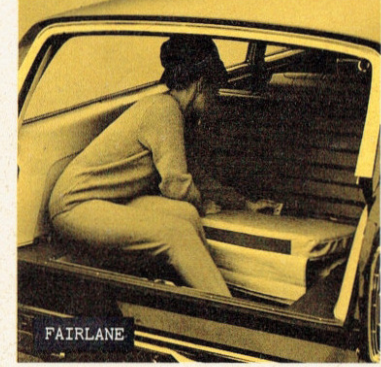
FAIRLANE 3. Next, seat-back cushion is positioned and snapped into place along its bottom edge.
