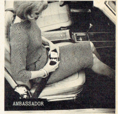
AMBASSADOR Auto-Lock belts, optional on all AM bucket seat models, except American, readjust automatically each time they're used. Retractor stores outer buckle, console pocket stores inner buckle.
