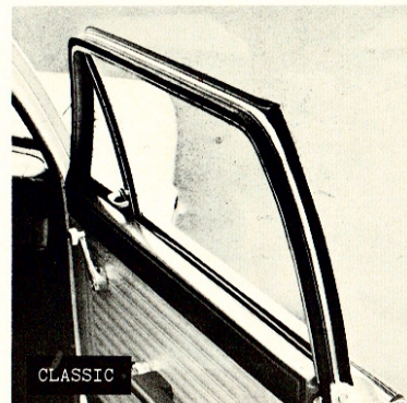
CLASSIC Double upper door seal on this Classic sedan (and all other AM sedans and wagons) forms a more reliable barrier against wind noise, especially important since upper door areas are close to passengers' ears.
