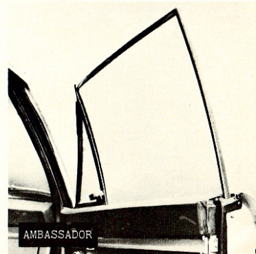
AMBASSADOR Framed side windows are found on all American Motors/Rambler and Ford Motor hardtops and convertibles. Framed side windows seal better and protect the vulnerable glass edges from damage.
