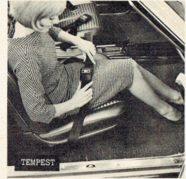
TEMPEST This Tempest model shows common problem of standard front seat belts: Awkward readjustment necessary for different-sized passengers. However, optional belt retractors do permit neat outer buckle storage.
