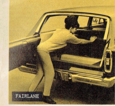
FAIRLANE Setting up the Fairlane (and the Comet) third seat is a four-step sequence. 1. First, the floor panel is opened and the seat back raised into position.
