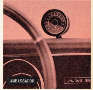
AMBASSADOR The AM tachometer (optional) is on top of the instrument panel where the driver can read it practically without taking his eyes off the road. A full 270-degree scale, also, improves readability.
