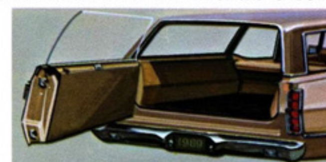
METEOR 3-WAY TAILGATE DROPS LIKE A TAILGATE, OR OPENS LIKE A DOOR WITH THE GLASS UP OR DOWN.
