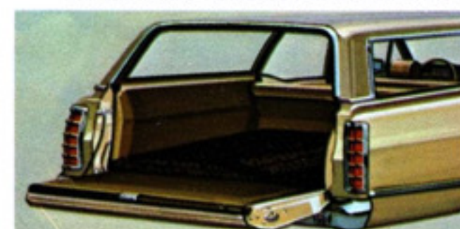
METEOR 3-WAY TAILGATE DROPS LIKE A TAILGATE, OR OPENS LIKE A DOOR WITH THE GLASS UP OR DOWN.
