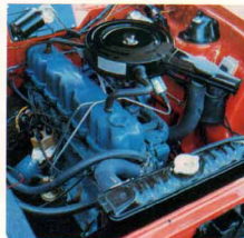
Economical 232 CID 6-cylinder engine
