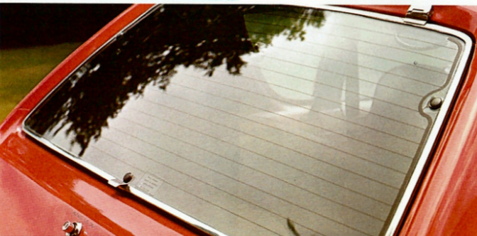
Rear window defogger. Keeps window glass frost and fog-free. (Larger alternator, tinted glass included as part of this option.)
