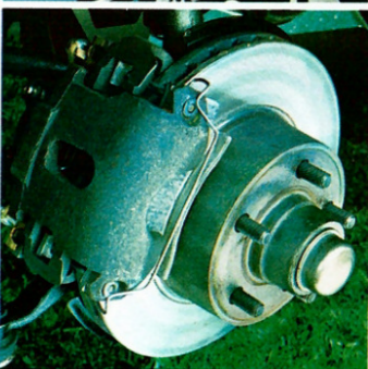
Power front disc brakes. Greater resistance to fade in repeated hard-braking situations with easier application.
