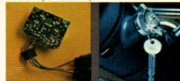
Solid-state ignition doesn't require breaker point replacement
