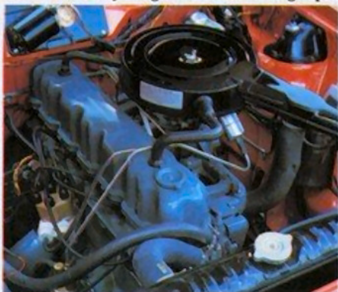
232 CID six (Pacer, Gremlin, Hornet)
