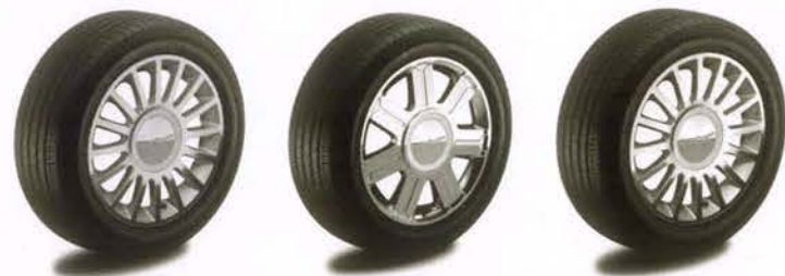
17" 16-Spoke Painted Aluminum Wheel Standard on Deluxe 17" 7-Spoke Chromed-Aluminum Wheel Standard on Premium 17" 16-Spoke Micro-Machined-Aluminum Wheel Optional on Premium
