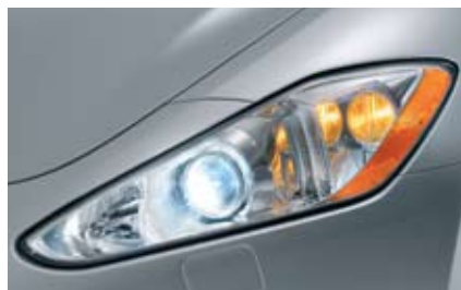
Bi-xenon headlights with headlight washing system
