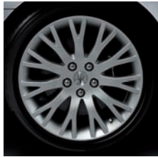
Light alloy wheels 18" (8.5J x 18" front; 10.5J x 18" rear) Standard on Quattroporte
