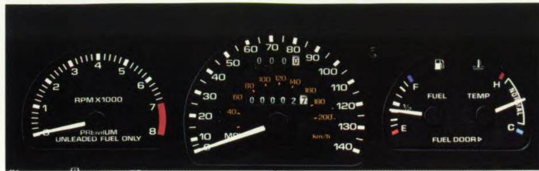
▲ Taurus SHO has a standard diagnostic instrument cluster with 8000-rpm tachometer.
