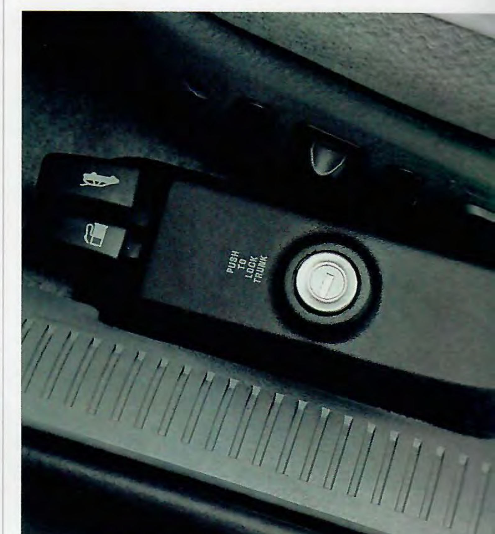
A remote liftgate release is now available along with the fuel filler door release in the wagon model.
