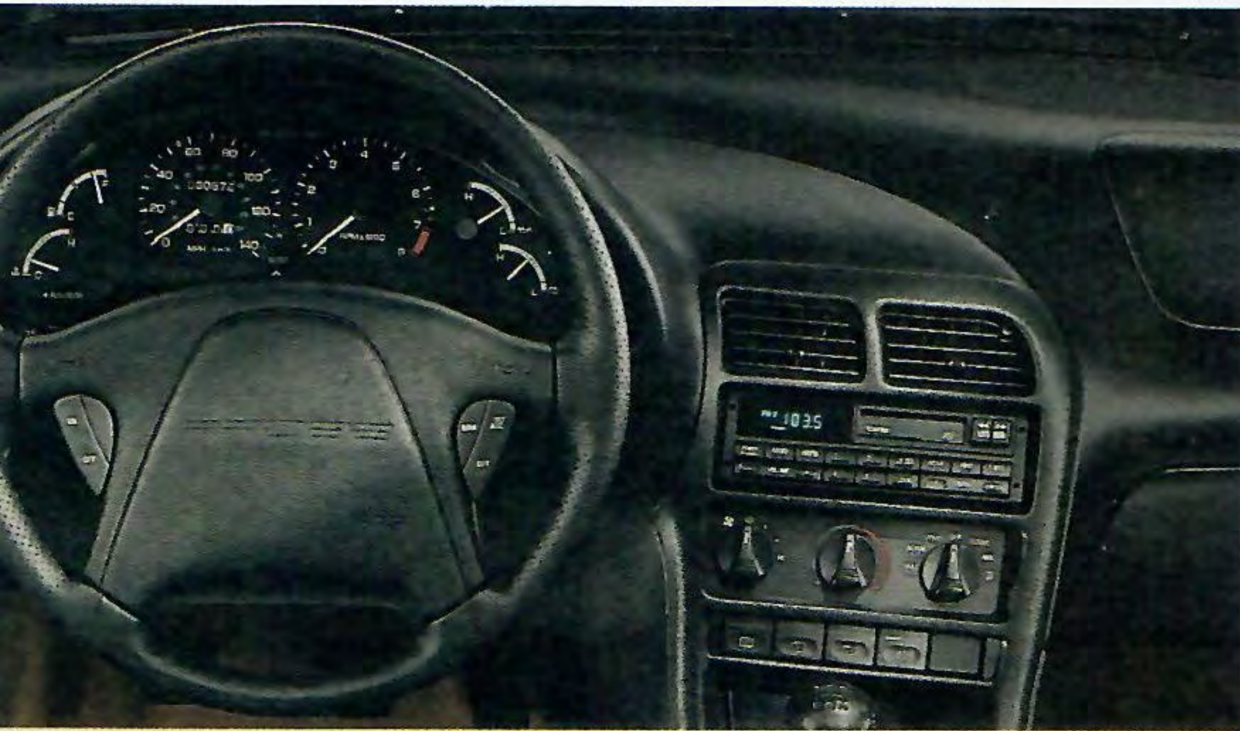
Probe's performance instrumentation includes a tachometer, temperature gauge, oil pressure gauge and voltmeter.
