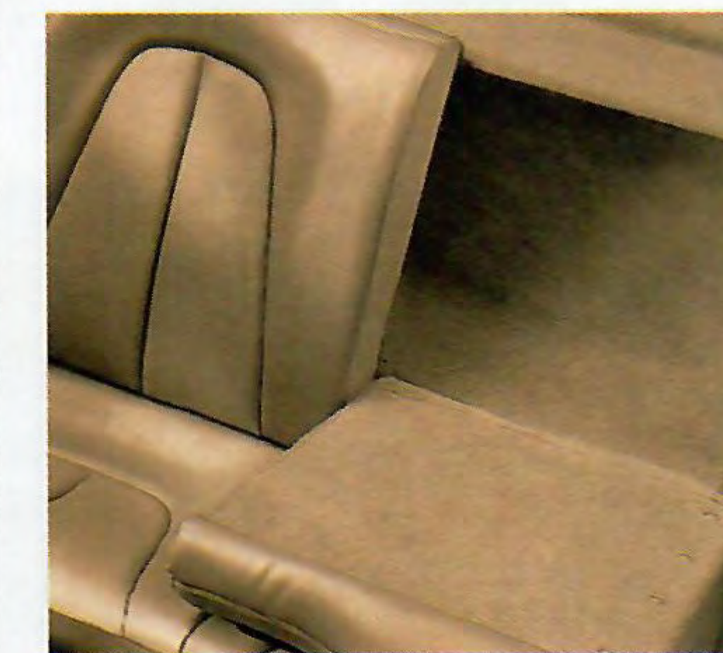
50/50 SPLIT REAR SEAT BACKS can be lowered individually, allowing for added cargo, with or without a third passenger.
