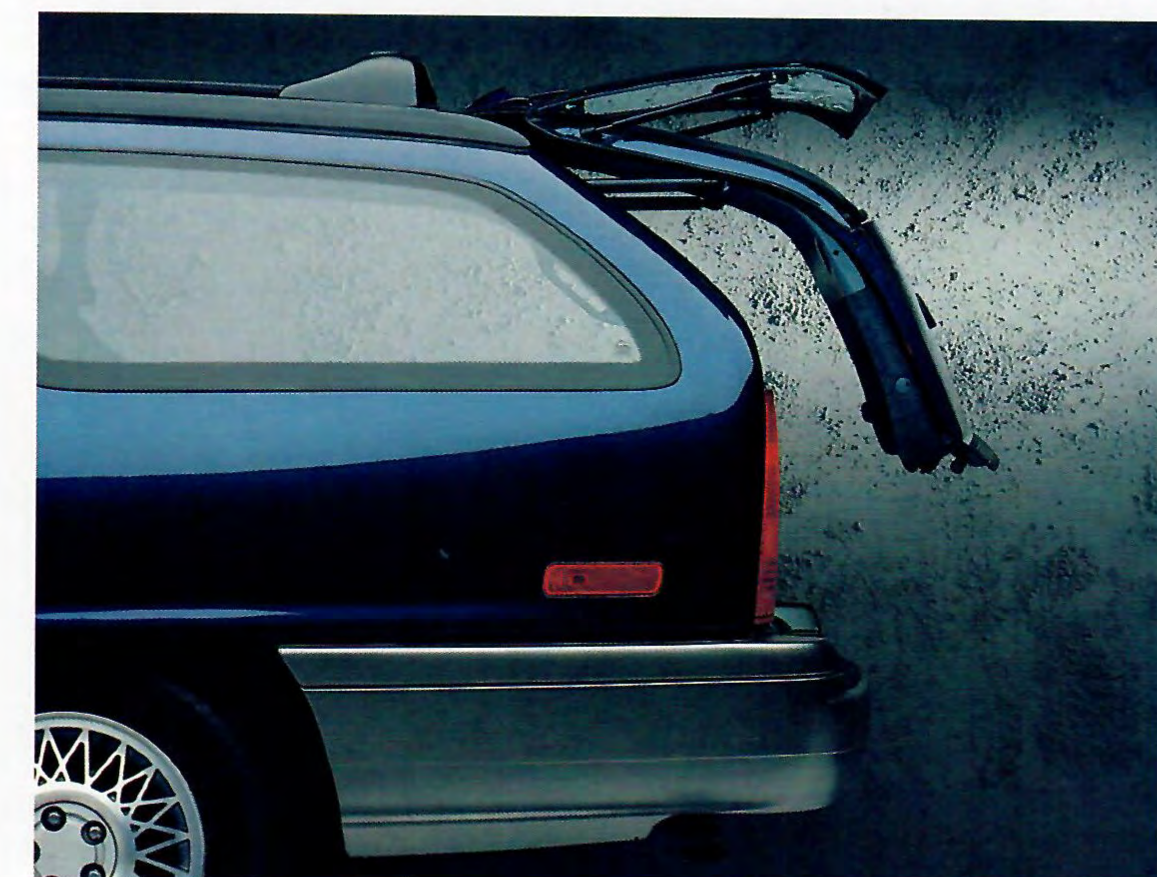
Liftgate features flip-up window for handy access to the rear cargo area without lifting the entire liftgate.
