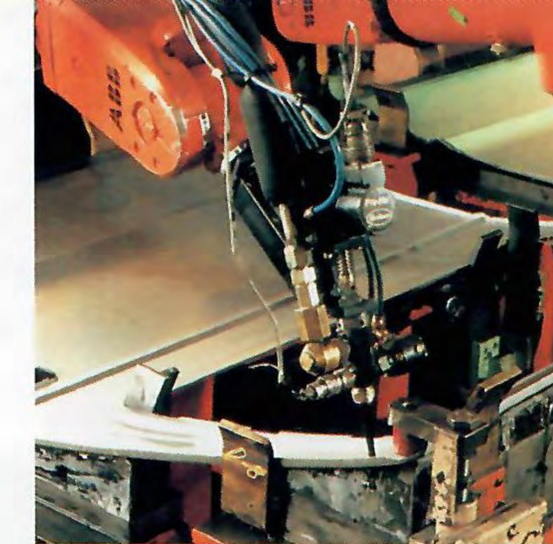
"Anaerobic" bonding of the inner to outer door assembly offers reduced noise and improved corrosion resistance.
