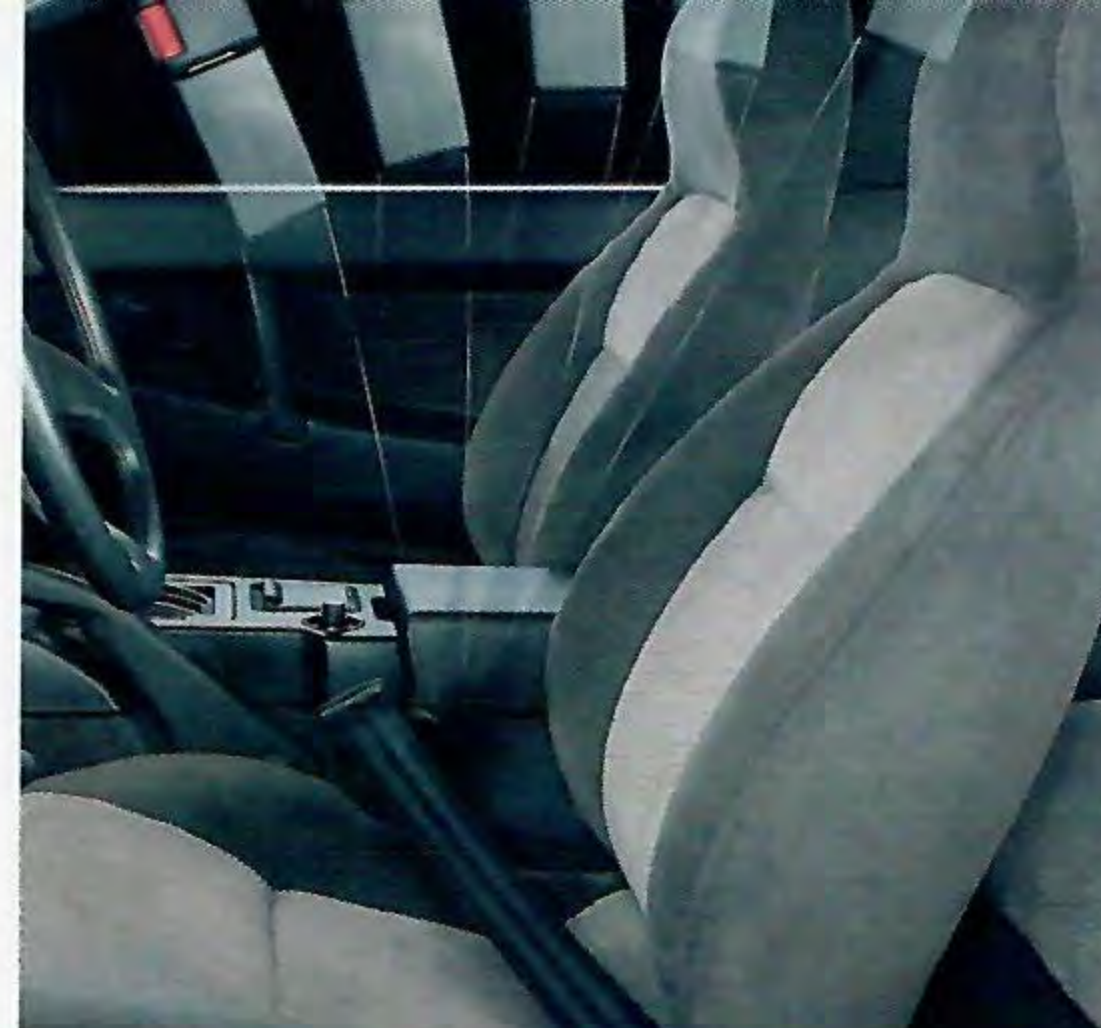
Front motorized passive restraints with manual active lap belts and rear lap/shoulder belts hold occupants safely.
