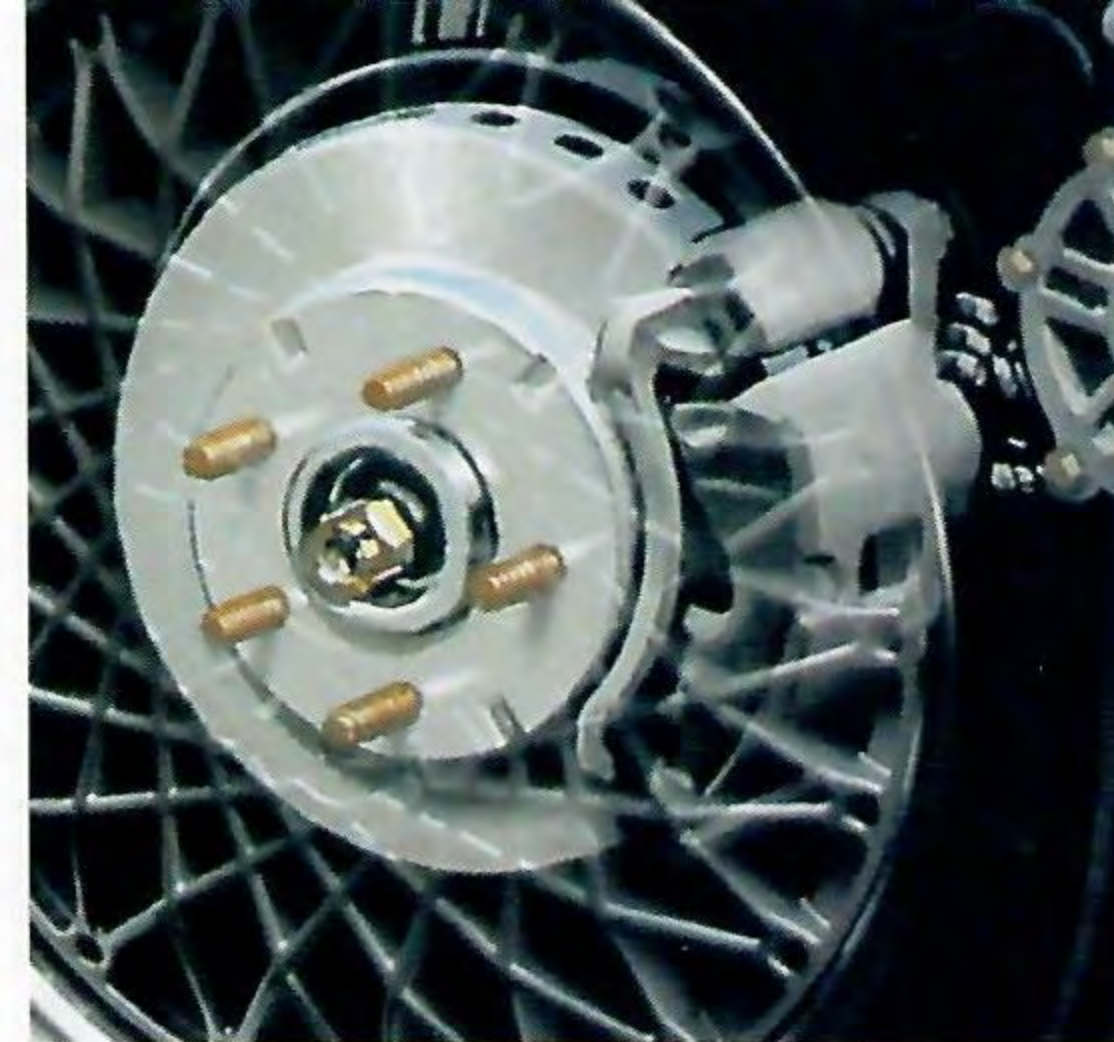
Four-wheel antilock brakes help prevent wheel lockup. (Available on Laser RS, RS Turbo, and RS Turbo AWD.)
