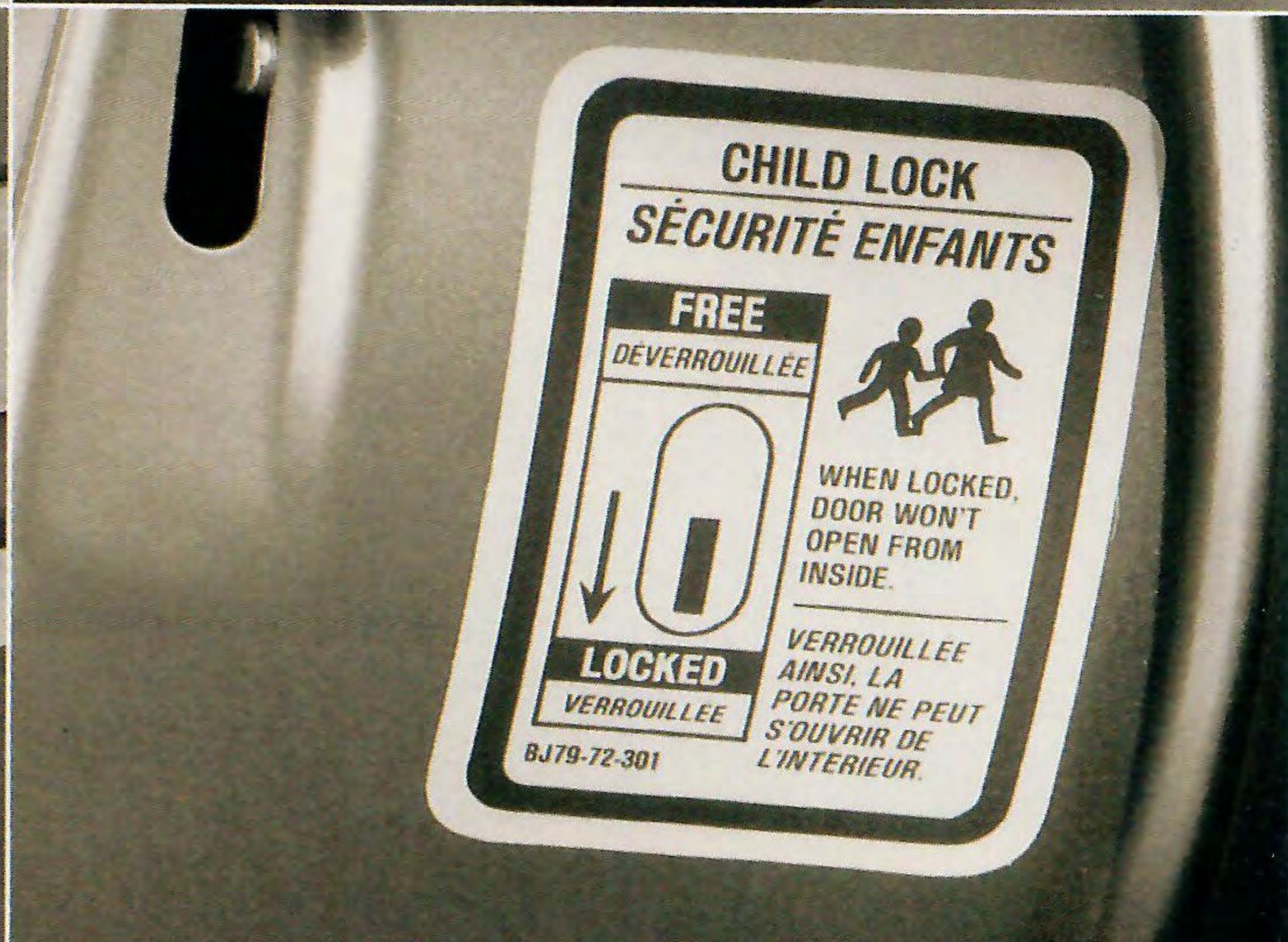
Child-proof door locks in the rear doors of all Mercury sedans as well as Villager keep children in back from accidentally opening the doors from inside the car, while allowing parents to still open doors from the outside.
