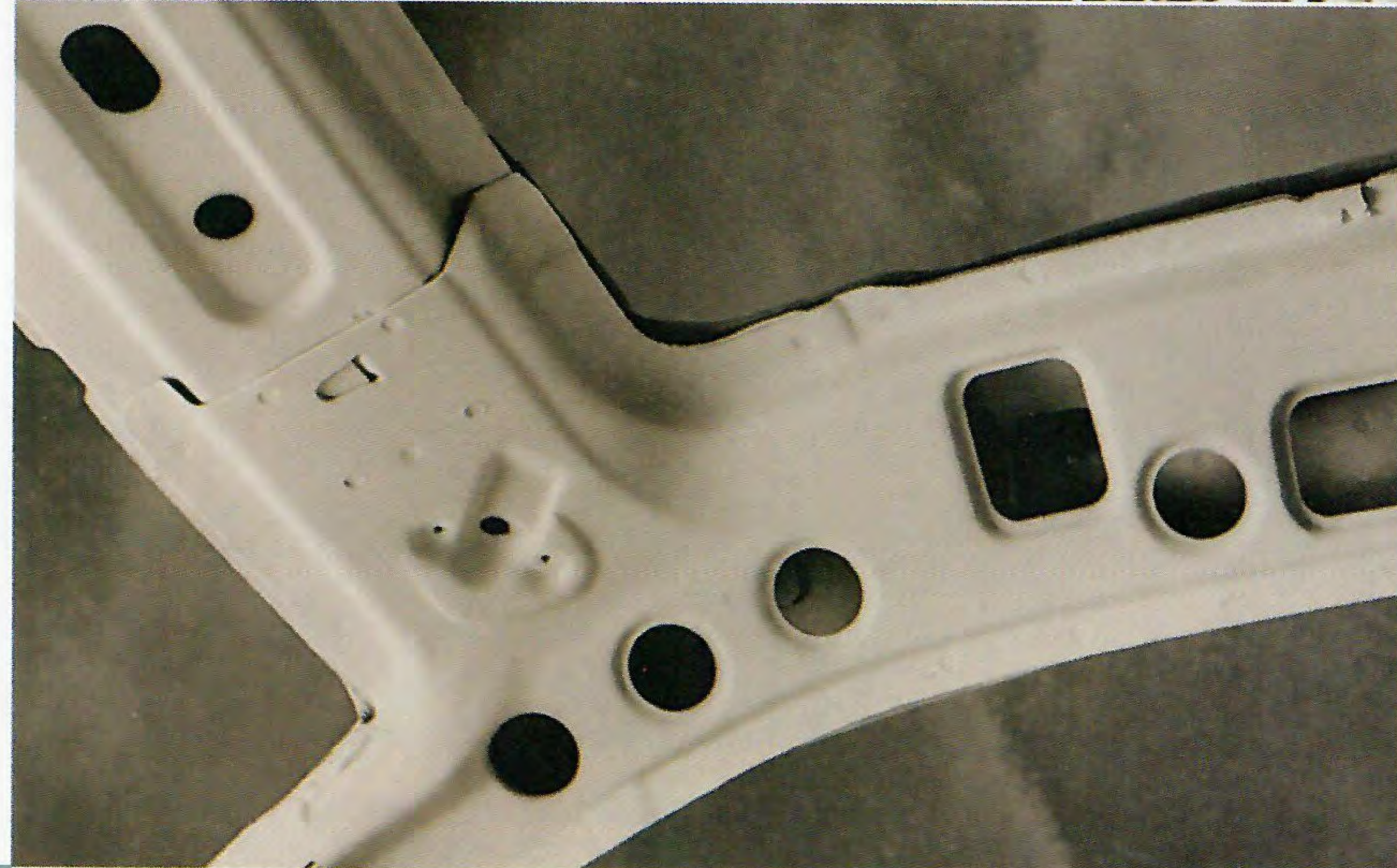
For protection in a rollover accident, the front pillars and the roof of every Mercury hard top are specially reinforced to withstand a static force roof crush test equal to to 1½ times the vehicle's weight.
