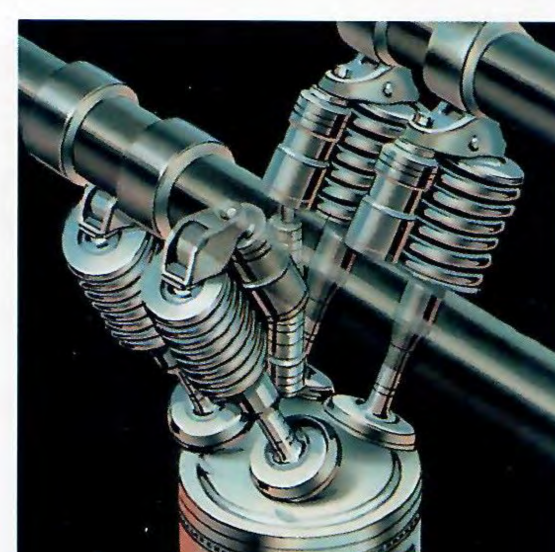
Four valves per cylinder offer high output and smooth performance on Laser RS, RS Turbo, and RS Turbo AWD.
