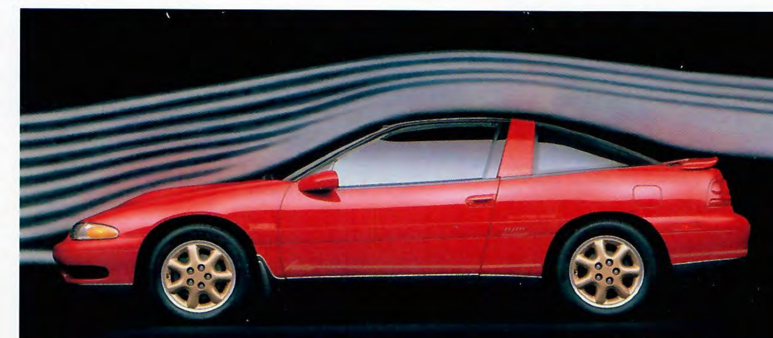
Base Laser's sleek and aerodynamic shape has earned an impressive drag coefficient of 0.33. A rear spoiler with integral center high-mounted stoplight is standard on Laser RS, RS Turbo, and RS Turbo AWD models, available on base Laser.
