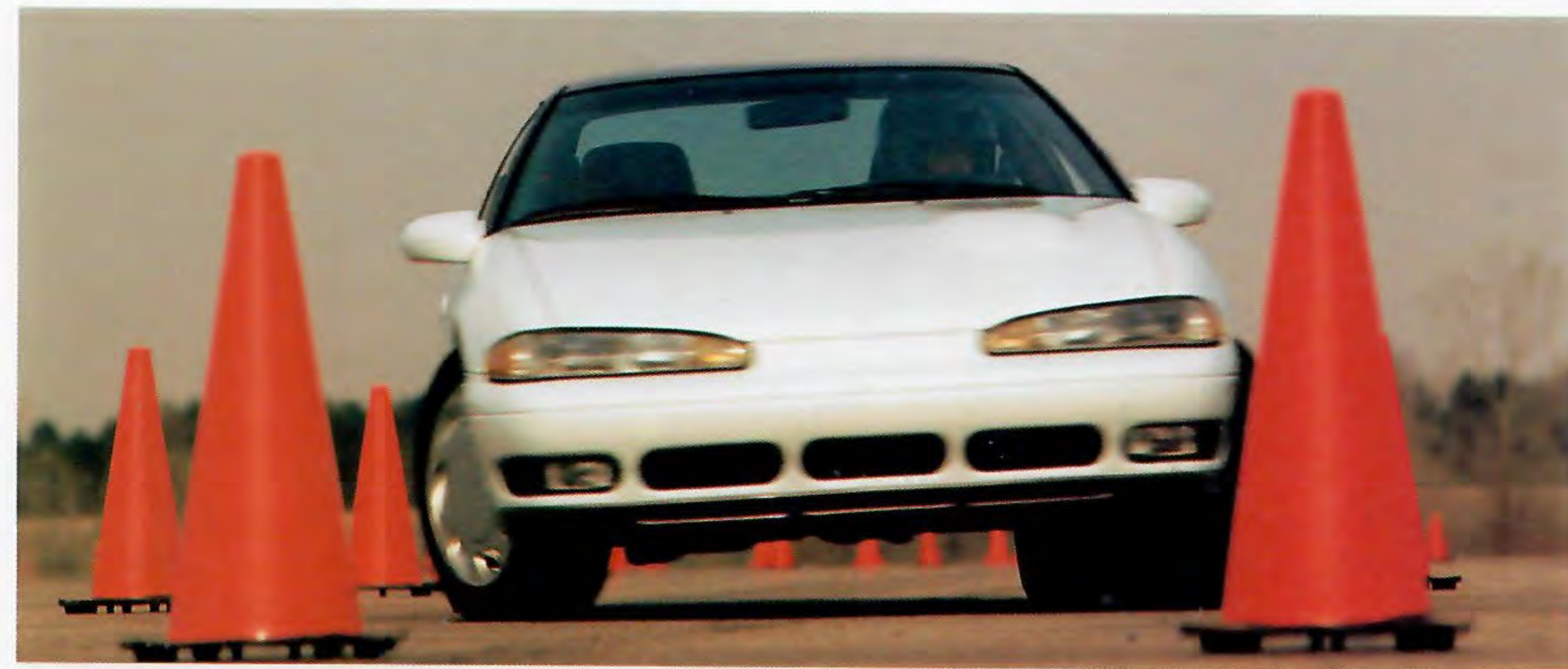
15.8:1-ratio power-assisted steering provides quick, responsive handling and a firm feel of road surfaces. (Optional on base Laser, standard on all other models.)
