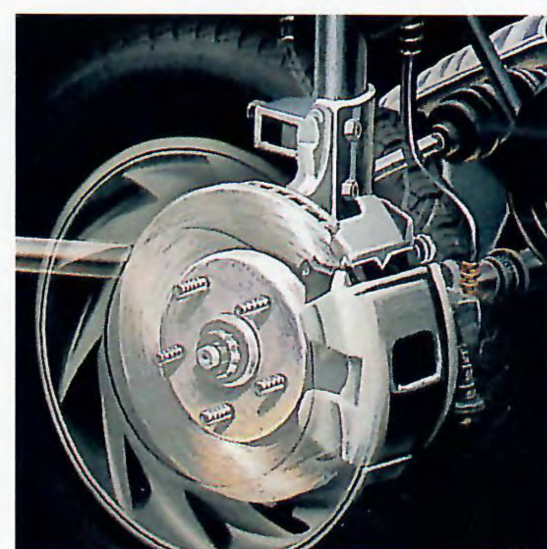
New for 1993, a vacuum-boosted antilock disc brake system is available on all Duster and Sundance models for increased stopping power.
