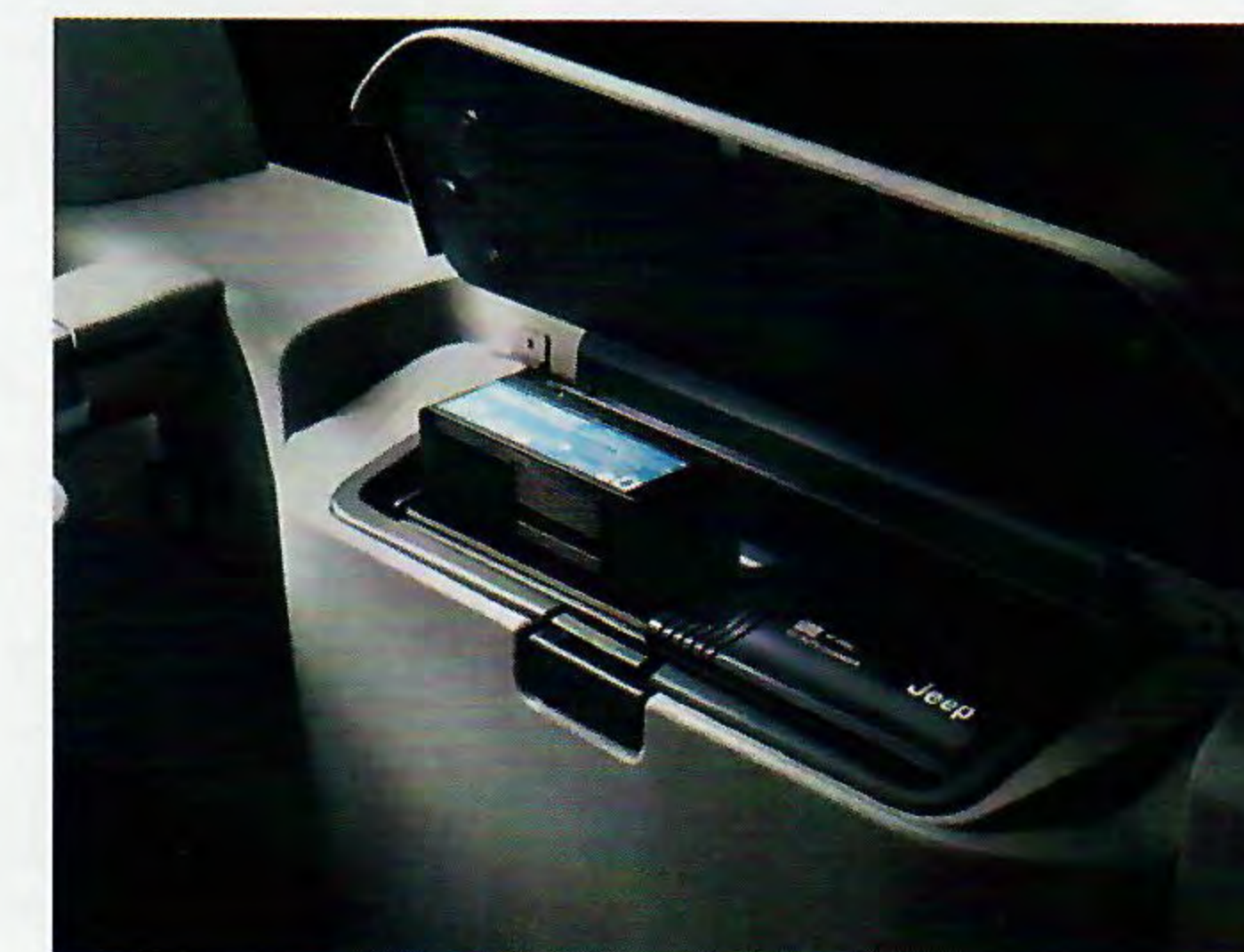
New for 1999, Grand Cherokee's cargo area provides room for an optional CD changer with 10-disc capacity that's mounted in a covered compartment on the right cargo area trim panel.
