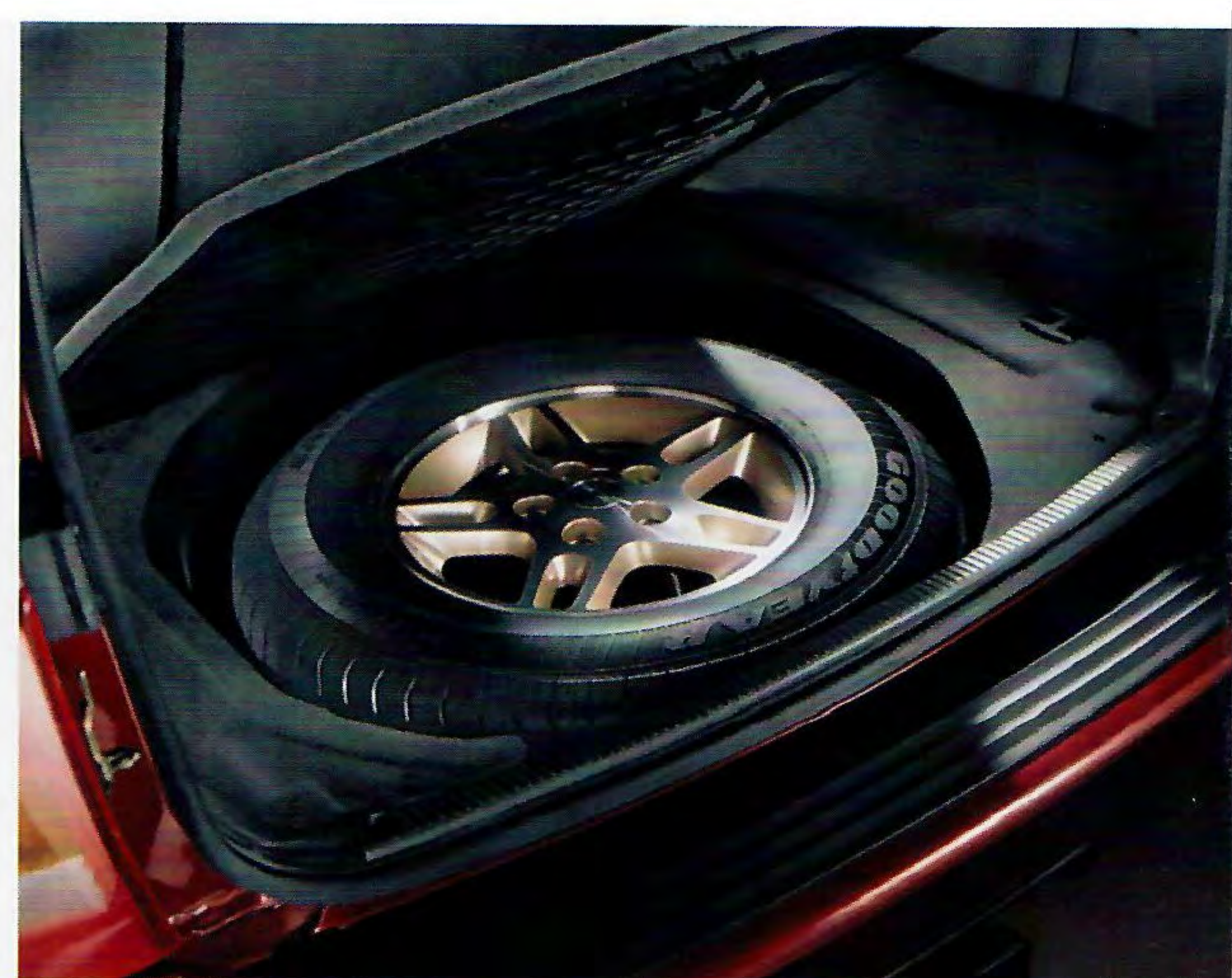
A removable lid that rests flush with the surrounding rear load floor covers the spare tire well, while a molded seal at the rear minimizes transfer of road noise into the interior.
